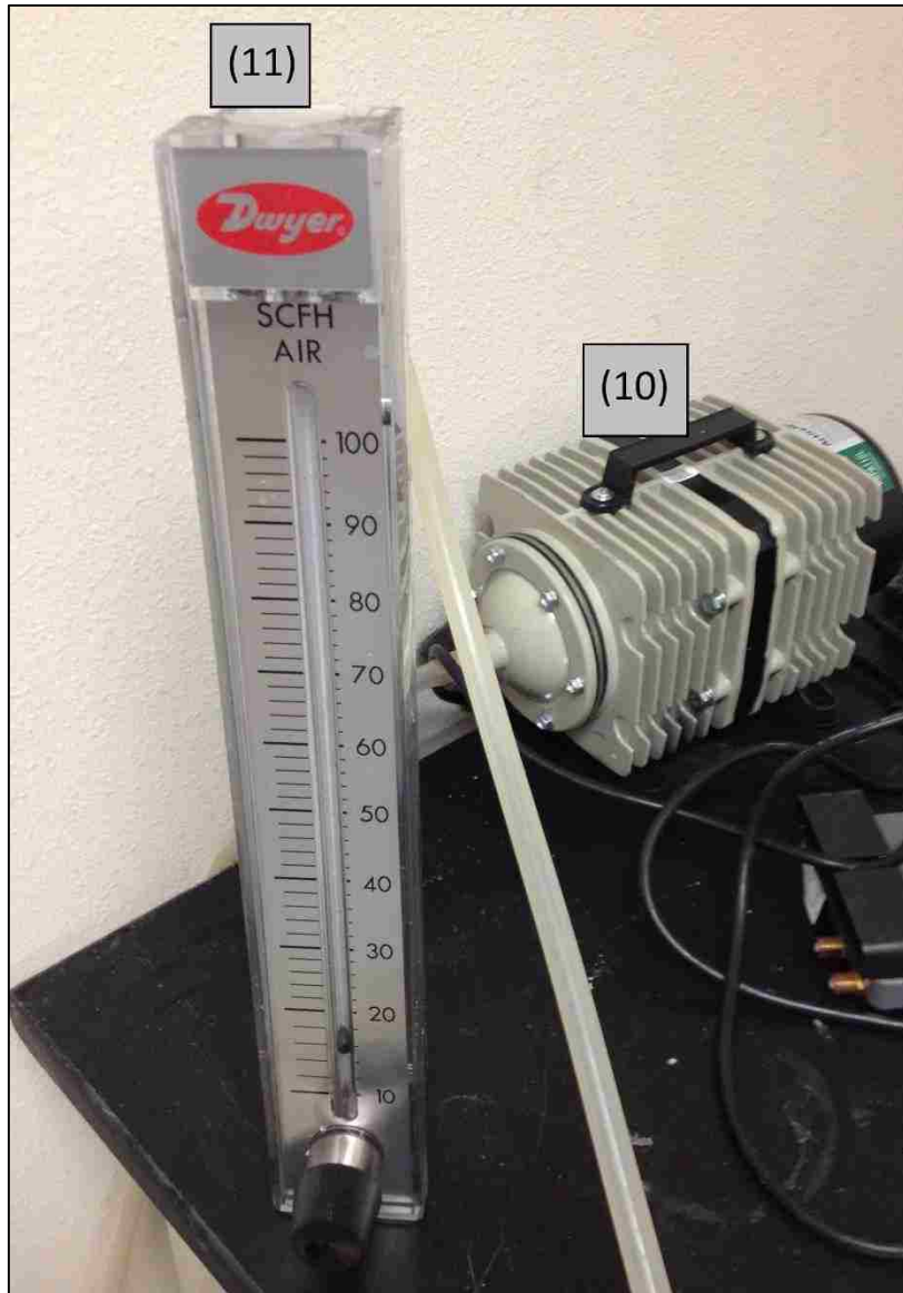
Figure 12 – Air flow and control for coarse bubble mixing.
