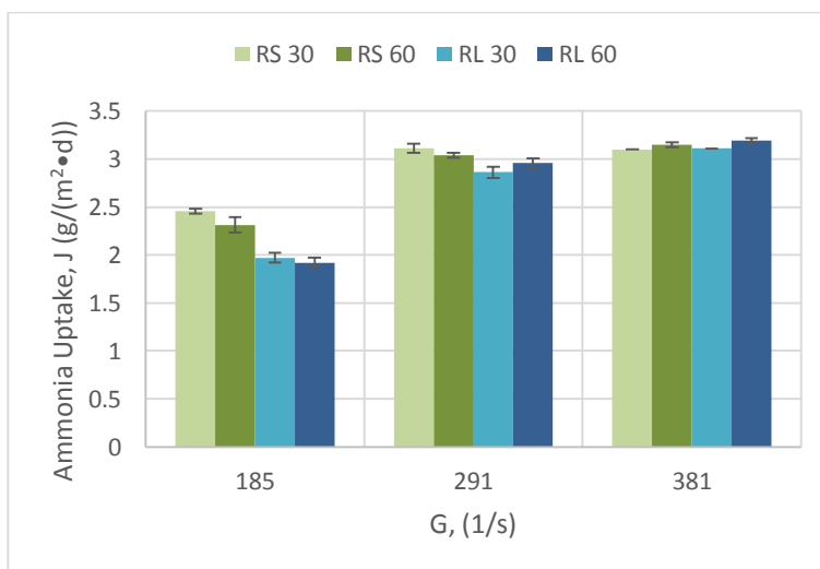
Figure 24 – AOB activity of R-Short and R-Long during 30 mg N/L and 60 mg N/L batch tests; error bars show ranges.
